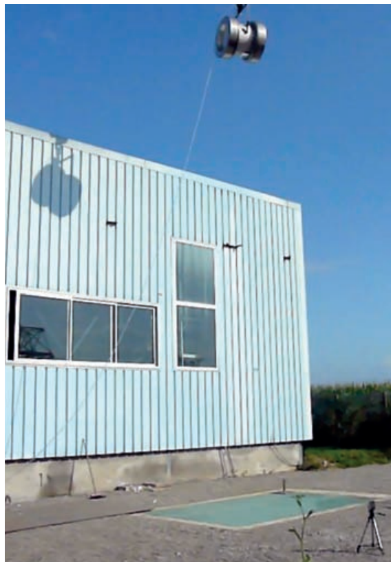
Package model undergoing 9-m free drop test
