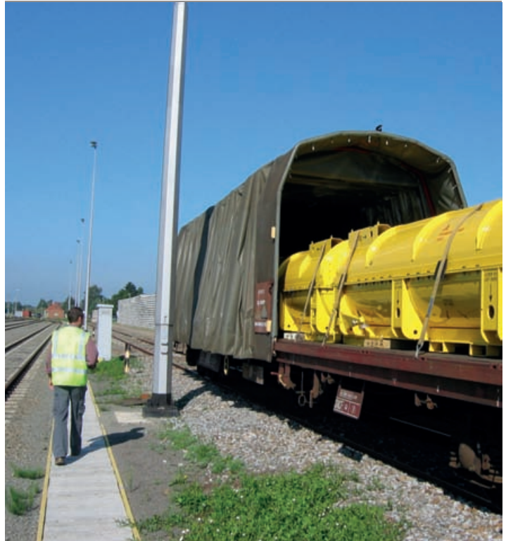
FCC packages intended for the transport of fresh fuel
