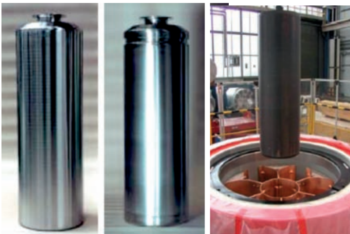
Vitrified waste canister (CDS-V)
